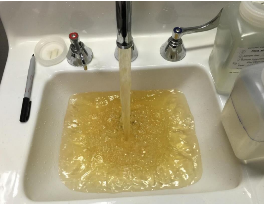
2015: Flint River without Corrosion Control
